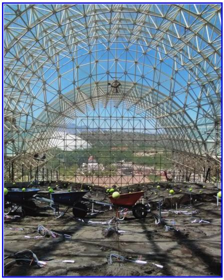
One of the three large "landscapes" that constitute Biosphere 2's (B2's)Landscape Evolution Observatory. Dark volcanic soil covers the tilted platform. Sensors, their locations marked here by yellow tennis balls, will send data to B2's computers, where researchers can control inputs (rainwater, carbon dioxide, temperature) and measure the results. Photograph: Fred Powledge.
